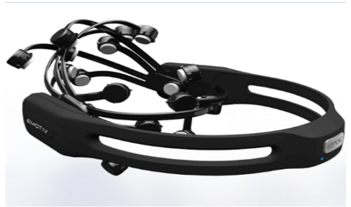
Fig. 1: EMOTIV EPOC+ headset: The EEG channels record the Electroencephalography activity and pass them for further processing and analysis.
